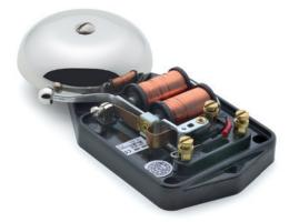
A Bakelite® housing that contains an electric ringing mechanism from the 1960s: our doorbells. With flat or cone ringer. These melodious items should not be connected to a power line, but to a bell wire with an upstream transformer (output voltage 8-12 V~).
