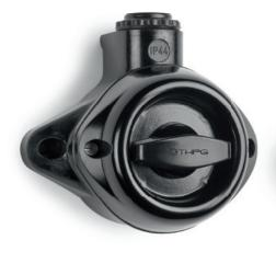
Rotary switch alternation moisture-proof 10 A, 10 AX, AC 250 V, IP44. 96 x 85 mm. Height above plaster 70 mm. Two-part case and handle made of Bakelite with a single input. Product code **100831**
